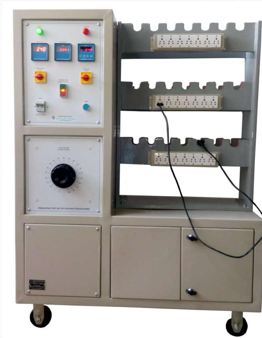
Preheating Test Setup For Hair Straightener
