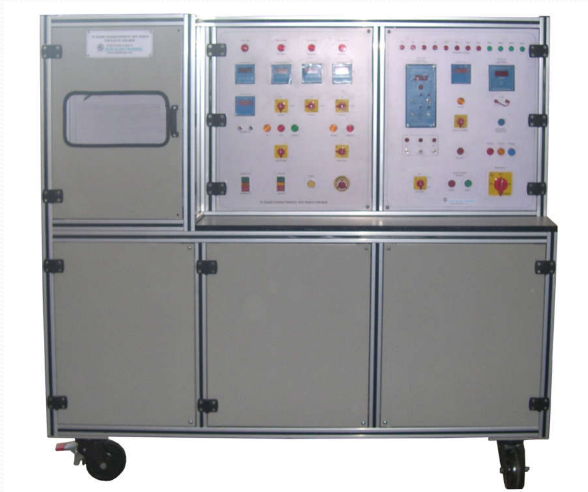
MCB Thermal + Magnetic Characteristic Test Bench
