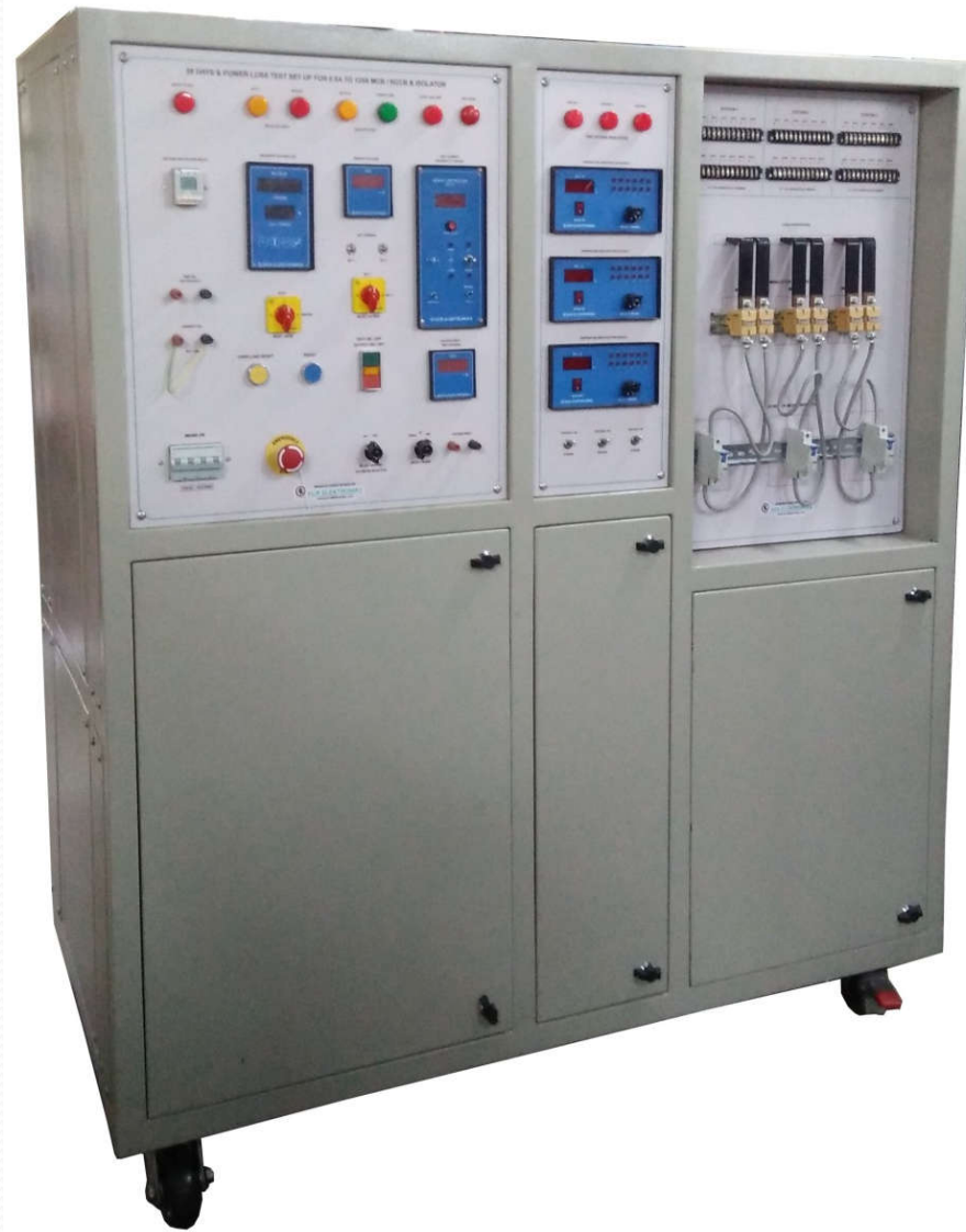
MCB 28 Days & Temperature Rise Test
