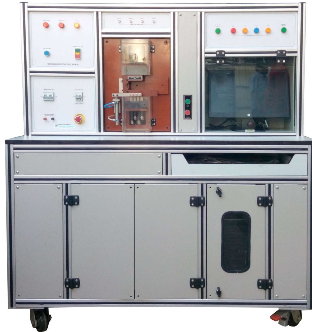
PC Based Fully Automatic MCB Magnetic Trip Test Bench
