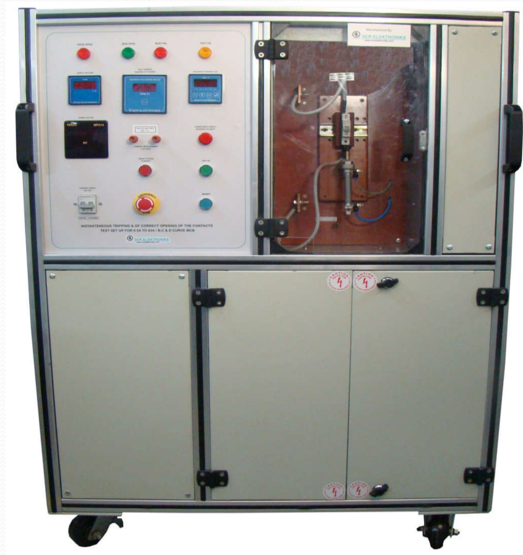
MCB Instantaneous Trip Test Bench
