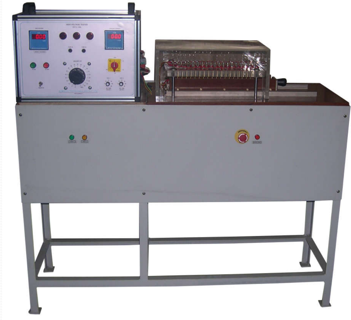
MCB 20 Station High Voltage Tster With Jig
