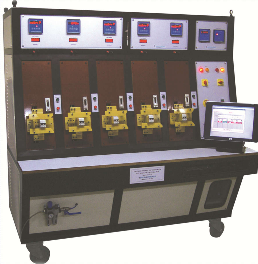
MCB Thermal Verification Test Bench
