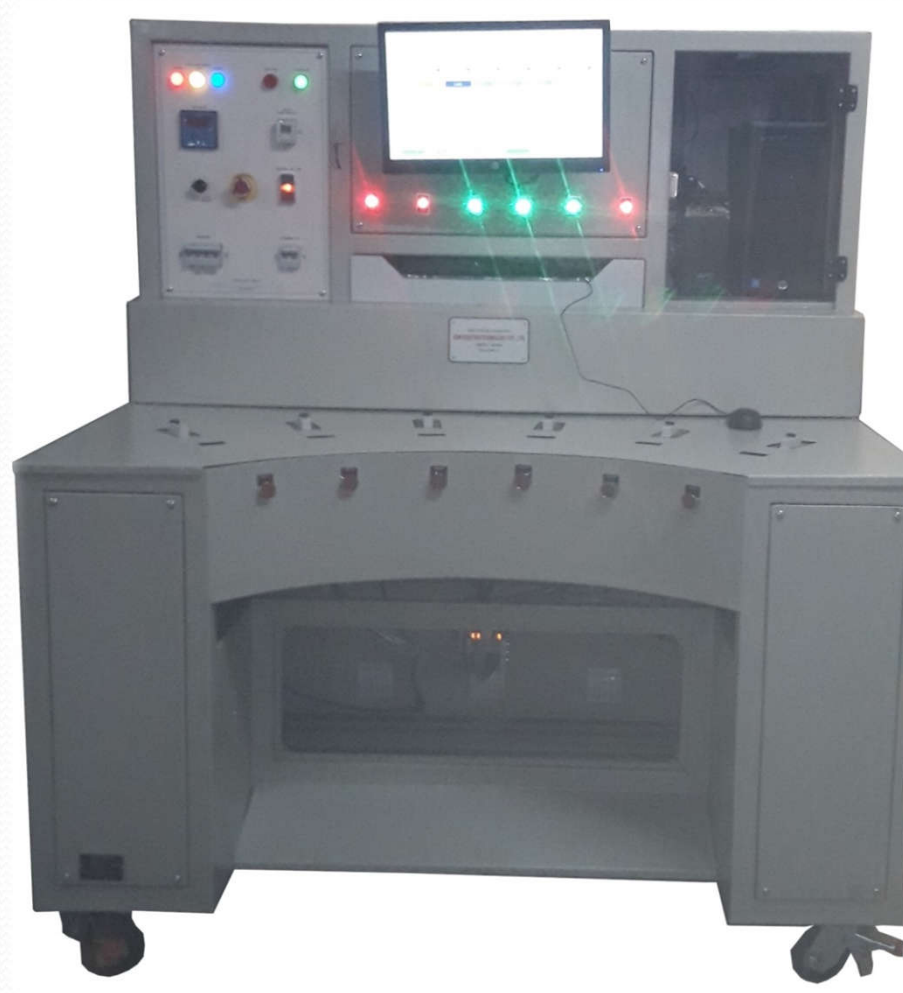
MCB Thermal Trip Calibration Test Bench
