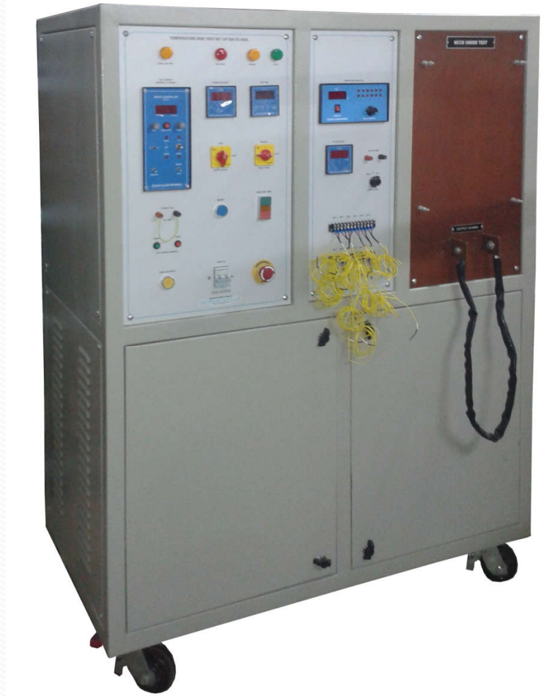
MCCB Temperature Rise Test Bench
