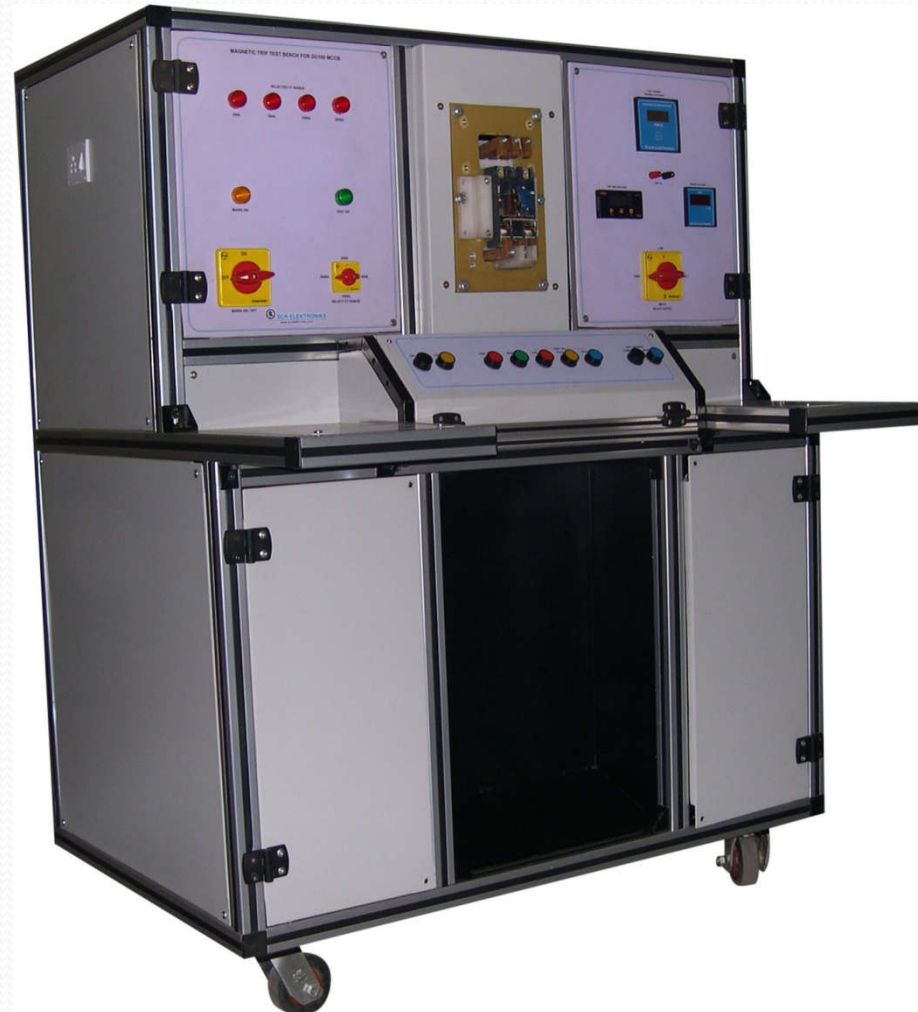
MCCB Short Circuit Trip Verification Test Bench
