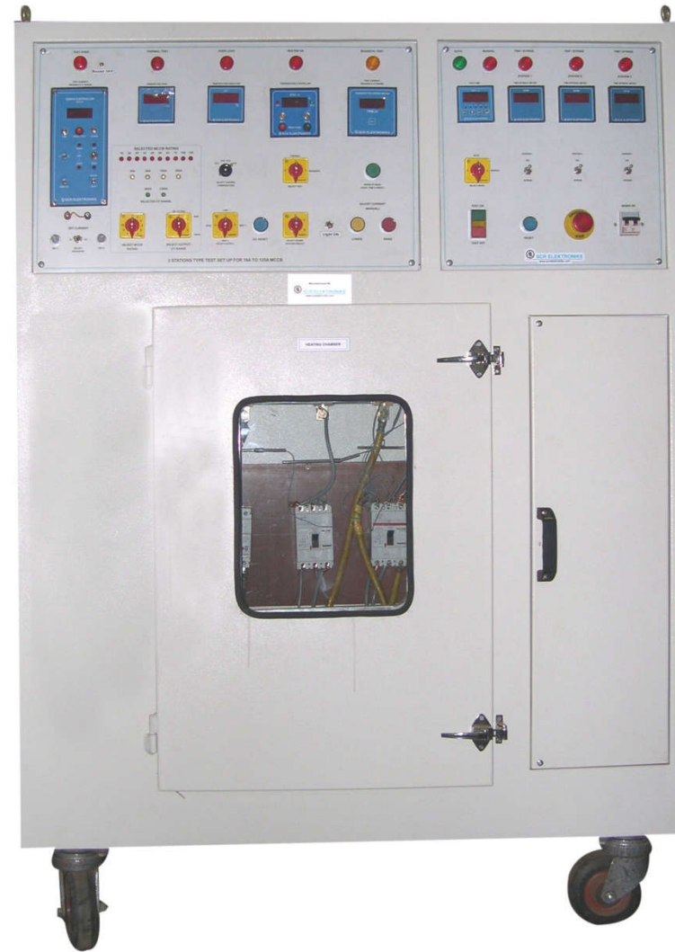
MCCB Audit Test Bench With Temperature Chamber
