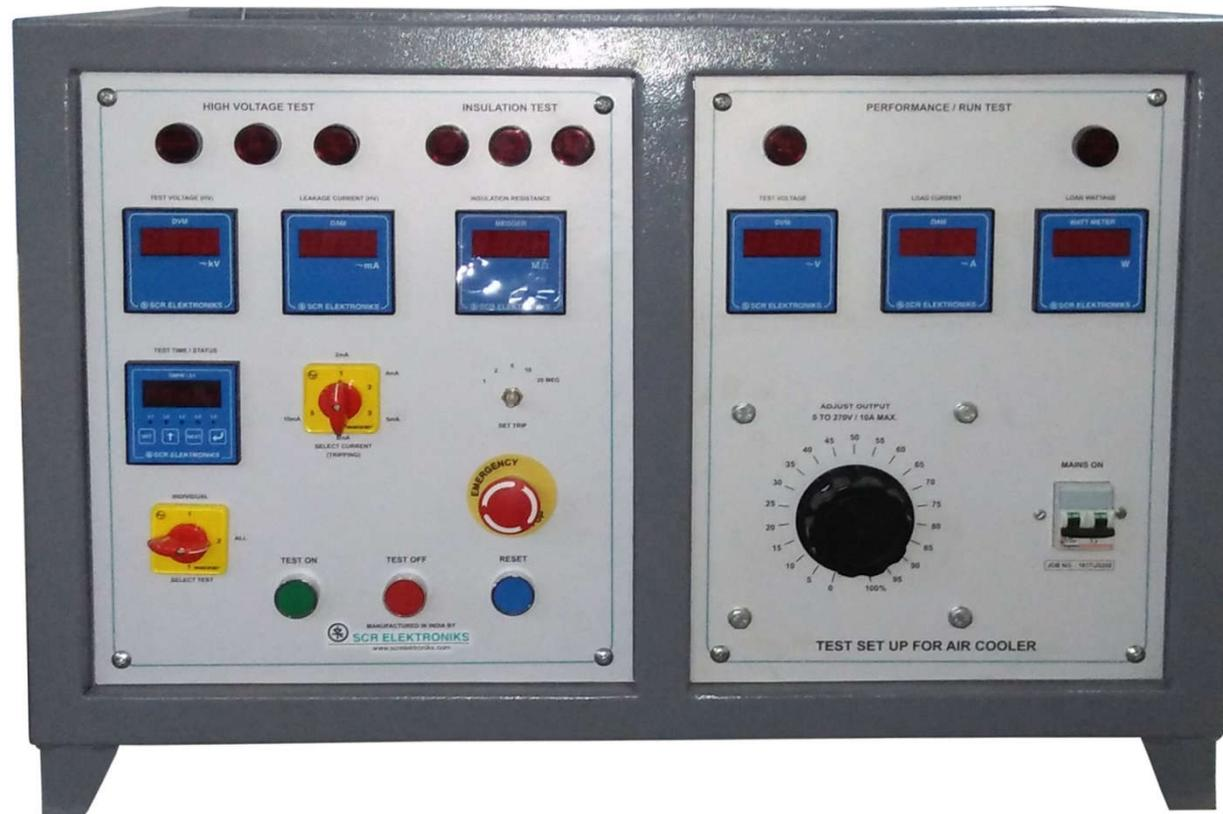
Test Setup For Air Cooler
