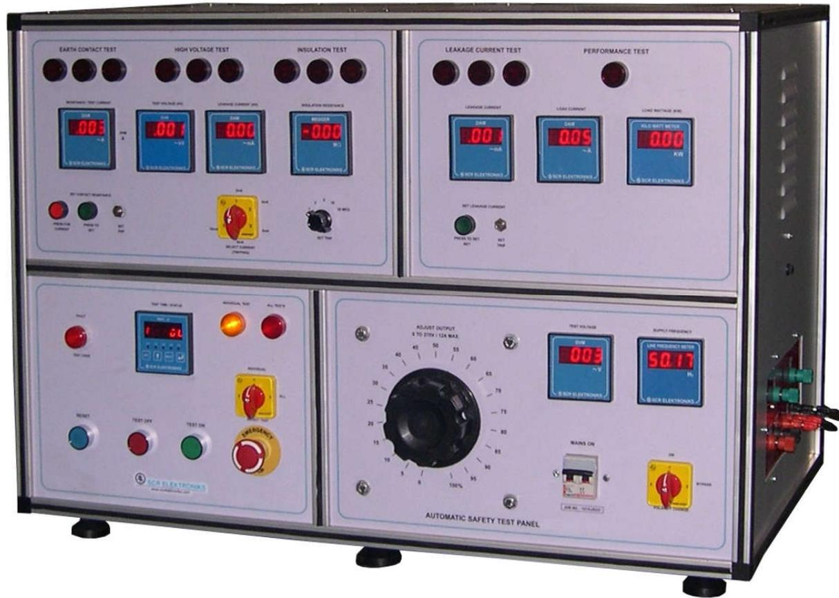
Automatic Safety Test Panel For Water Cooler
